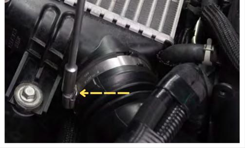
Loosen the clamp and remove charge pipe.
