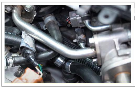
Step 51 Install the Y hose fitting onto block breather and push down.
