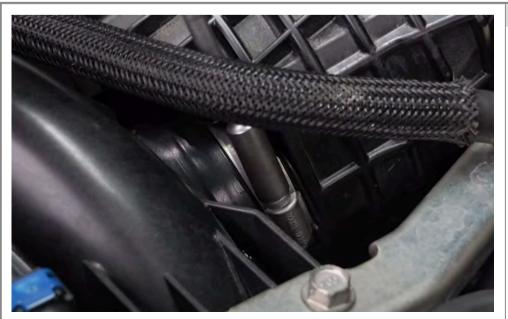
Step 82 Using a nut driver, tighten the throttle body clamp.
