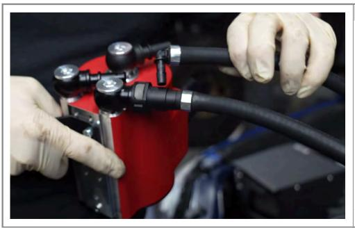
Note: These fittings are preinstalled and torqued. The fitting is designed to swivel around the bolt. Do not remove or tighten further.
