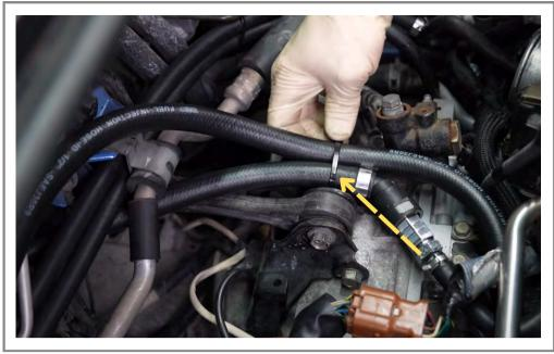
Step 55 Attach zip tie to hoses and tighten. Cut off excess zip tie.
