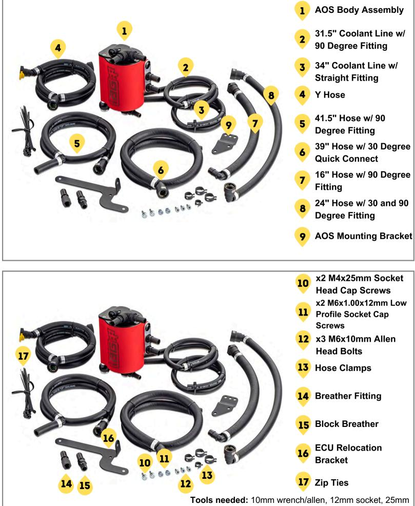
**Tools needed:** 10mm wrench/allen, 12mm socket, 25mm socket, 8mm nut driver, socket, razor, all purpose lube, needle nose pliers, pick tool, pipe/hose cutters, zip ties
