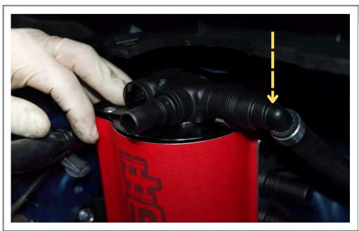
Step 48 Connect 90 degree fitting to top of AOS can.
