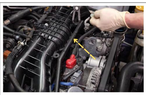
Step 59 Remove the two clips holding the PCV tube.
