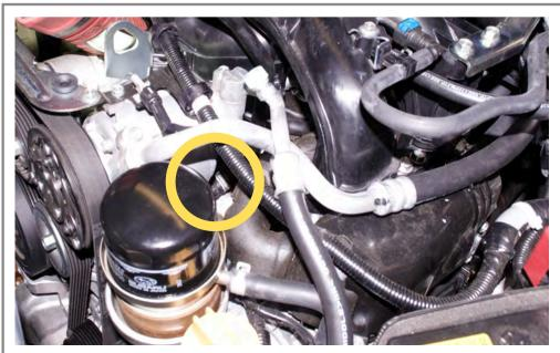
Step 57 With a pair of needle nose pliers loosen the clamp and disconnect the PCV hard tube.
