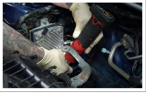
Remove the bolts holding the ECU to the bracket on the strut tower.
