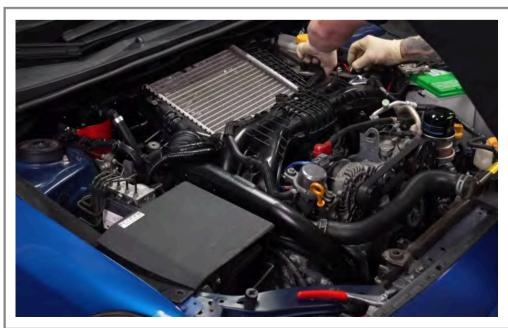
Step 79 Reinstall the top mount intercooler back on the engine.
