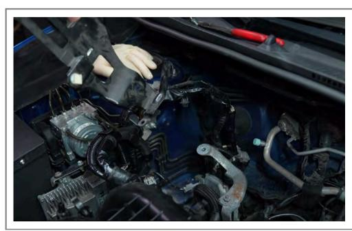
Step 27 Remove the two 10mm bolts which secure the ECU bracket to the strut tower.
