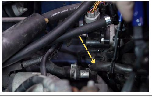
Loosen clamp and remove OEM coolant line.
