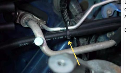
Using two zip ties secure the coolant lines to the AC hard line and brake master line.
