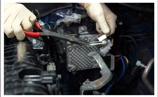
Step 24 Using pliers, remove the harness retaining clip from the bracket.
