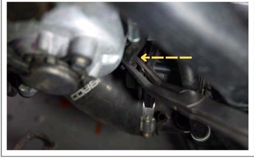
Using a pair of needle nose pliers, disconnect the bypass valve vacuum line.
