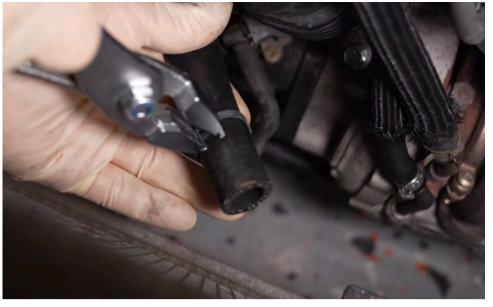
Use a pair of pliers to slide clamp onto hose.
