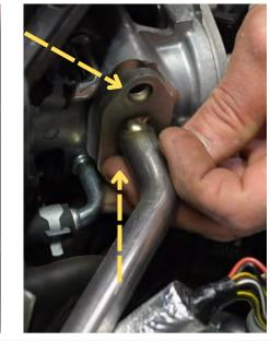
Remove the four 12mm bolts that secure the EGR pipe.
