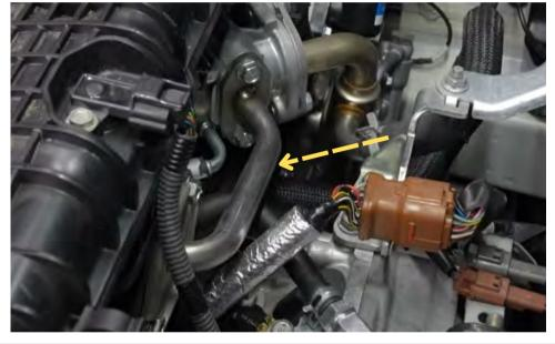
Reinstall the EGR pipe back to the manifold.
