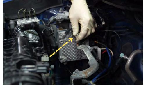
Remove the 10mm bolt securing the wiring harness to the ECU.
