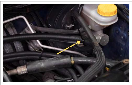
Step 65 Zip tie line to brake master line. Cut excess zip tie.
