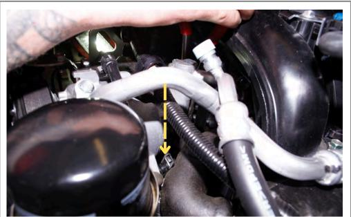
Step 62 Install the 90 degree fitting to the turbo inlet. Secure the clamp.
