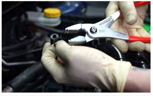
Slide a supplied clamp onto smaller coolant line.
