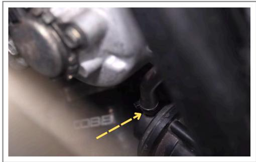
Step 67 Reconnect the vacuum line for the bypass valve.
