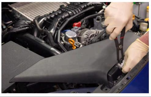
Remove the air intake duct by removing the two front clips.
