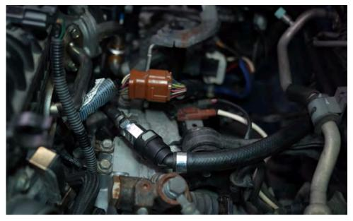
Connect the 30 degree fitting to the new breather fitting.
