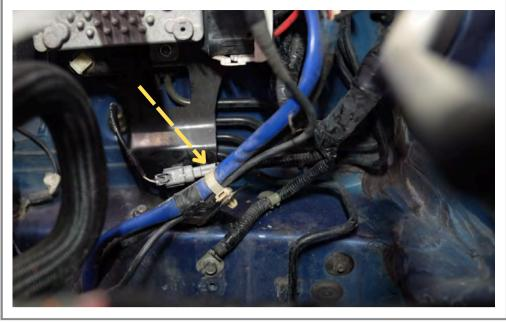
Using a pair of needle nose pliers remove the clip holding the harness in place below.
