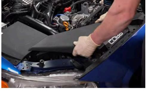
Reinstall the duct for the air intake using the plastic clips.
