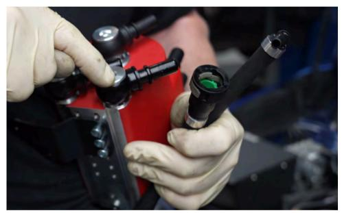
Step 35 Apply a small amount of lube to the coolant hose with the 90 degree fitting.
