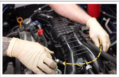
Step 61 Route the 90 degree fitting under the intake manifold.
