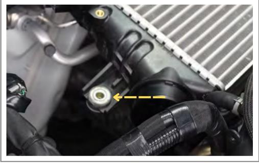
Remove the intercooler bolt on the passenger side with a 12mm socket.
