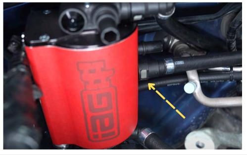
Connect the other end of the breather hose to the bottom port on the AOS.
