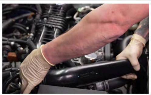
Step 66 Reinstall the charge pipe and tighten the top clamp.
