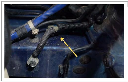
Use pliers to remove this mounting tie from the frame rail.
