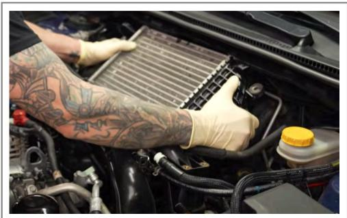
Step 12 Remove the intercooler by pulling up and away from the throttle body.
