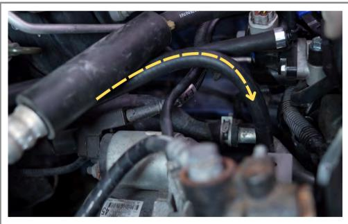
Step 42 Install new coolant line to OEM fitting.
