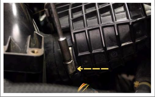
Loosen the clamp on the throttle body.
