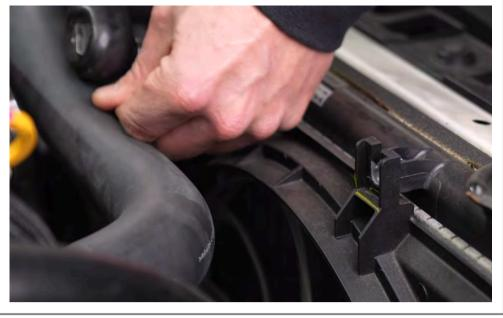
Unscrew the two bolts that secure the radiator fan.
