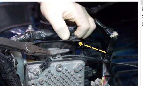
Step 21 Using a pair of needle nose pliers remove the clip holding the harness in place.
