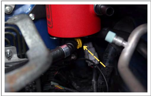
Step 54 Connect the drain hose to the bottom of the AOS can and press tab down to secure.
