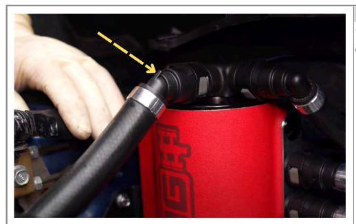
Step 73 Connect fitting to top of AOS can.
