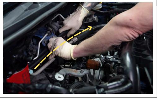
Route the two coolant lines behind the AC hardline.
