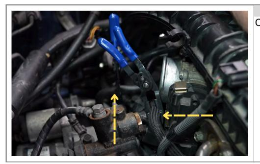
Step 40 Clamp both OEM coolant lines.
