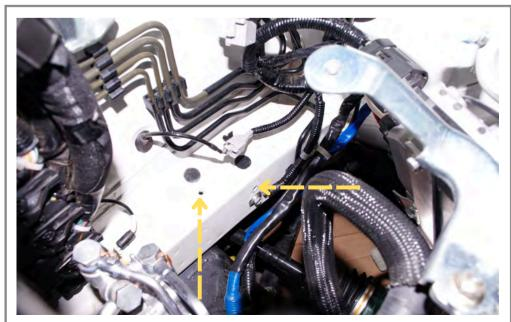
Step 30 Attach the ECU relocation bracket using the OEM ECU bracket 10mm hardware.
