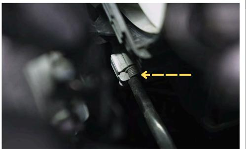
Step 3 Disconnect passenger side radiator fan wiring harness.
