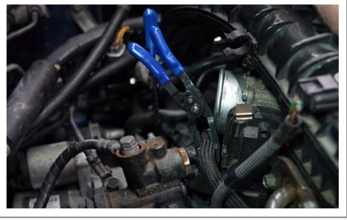
Remove both coolant line clamps from step 40.
