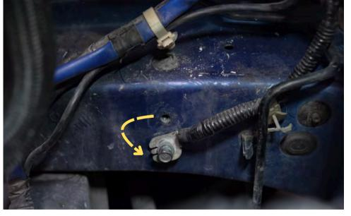
Reinstall the ground to this hole using the OEM 10mm bolt.
