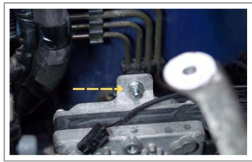
Step 32 Attach the ECU to the new bracket using the supplied bolts.
