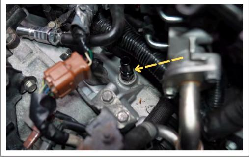
Install the new block breather and tighten to OEM specs.
