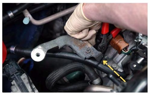
Step 56 Attach zip tie to drain line and bracket.
